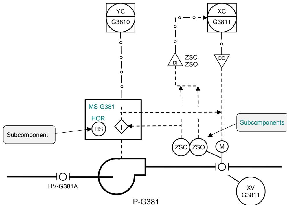
**Figure 7-5 : Subcomponents – Electrical and Instrumentation**
