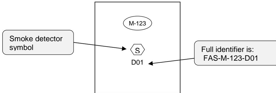
**Figure 6-5 : Room Numbering on Drawings – Plan View**
