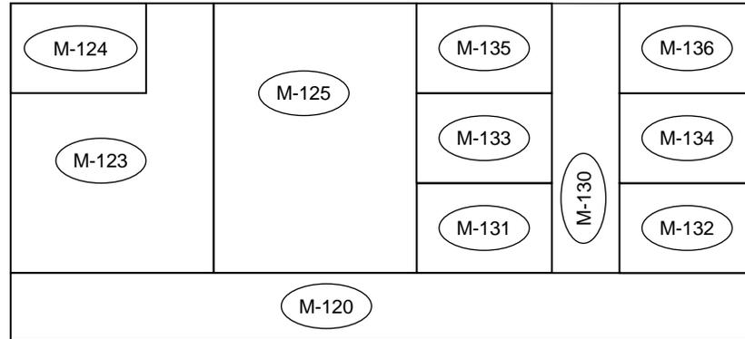
**Figure 3-1 : Room Numbering on Drawings – Plan View**
