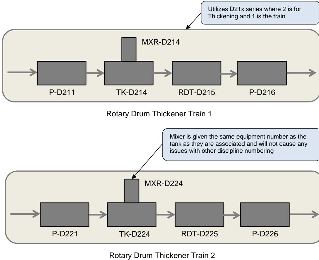
**Figure 2-2 : Sequential Logical Numbering Example**
