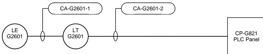
Figure 7-2: Instrument Cable Identification Example – Level Transmitter
