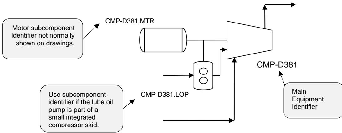
**Figure 2-3 : Lube-Oil Pump Subcomponent Example**
