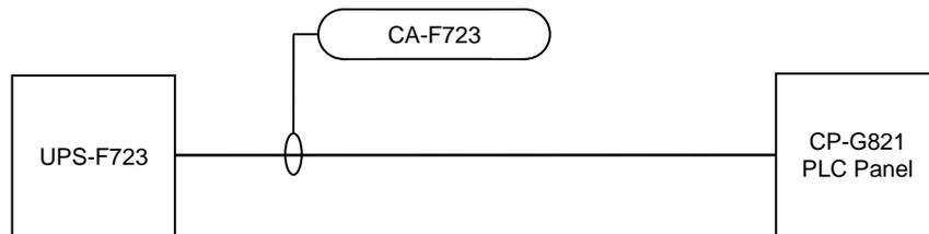
**Figure 7-3: Instrument Cable Identification Example – Identified Equipment**
