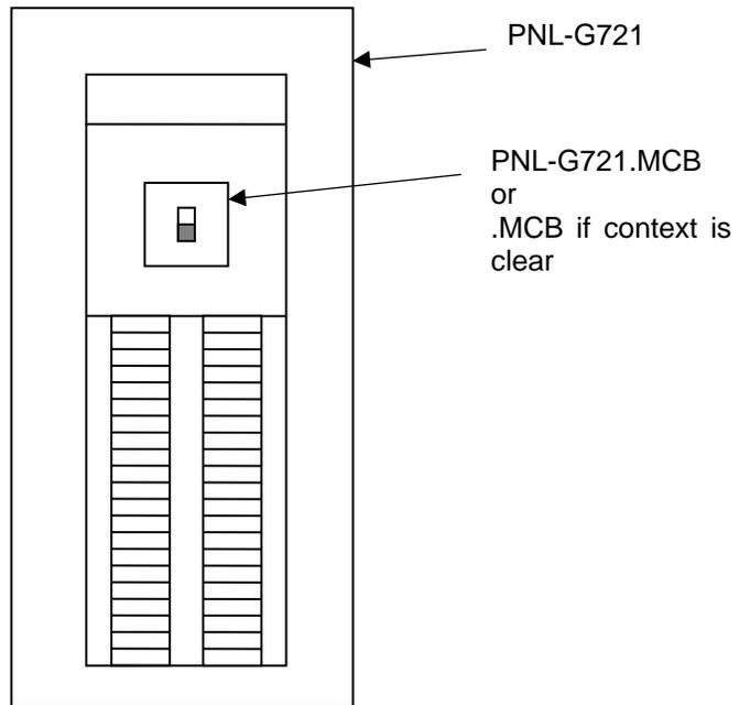
**Figure 2-4 : Electrical Subcomponent Example – Main Circuit Breaker**
