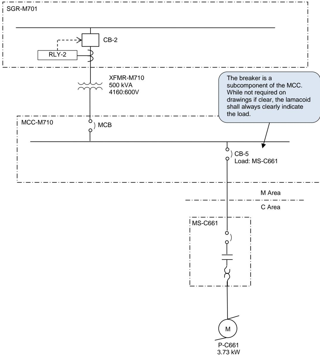
**Figure 6-4 : Example Identification by Load Equipment**
